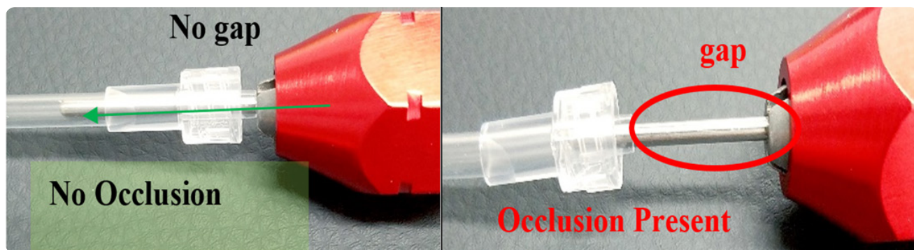
Figure 4. Go/No Pin fully inserted in non-occluded bond (left) and Go/No Pin partially inserted in an occluded bond (right)
